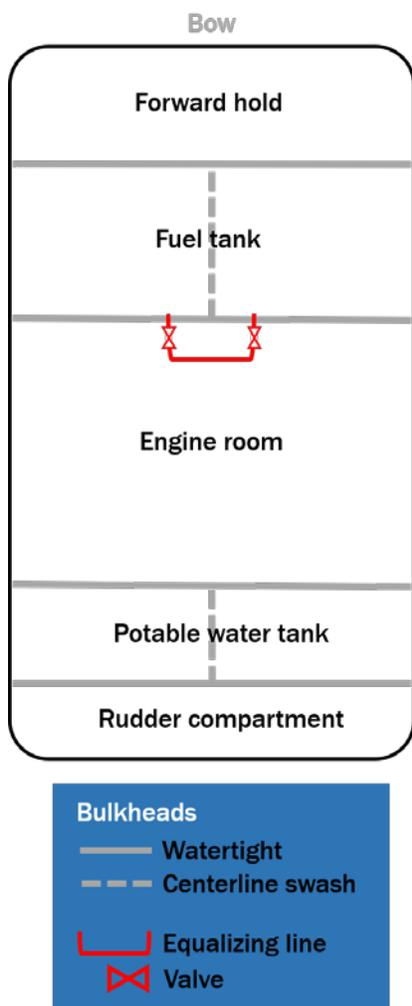
Plan view of *Gracie Claire's* hull, not drawn to scale. (Based on postaccident sketch by marine surveyor)
