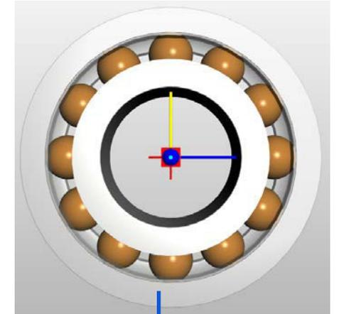
*QJ bearing replaced by nonlinear stiffness.*
