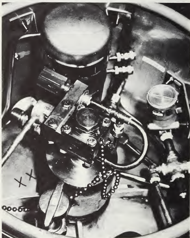
FIGURE 5.24. Top view of a 100-liter multi-shielded helium dewar showing ball valve access port, relief valves, and accessories.
