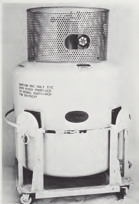
FIGURE 5.19. 500-liter vapor-shielded liquid helium dewar (Airco Cryogenics Division).
