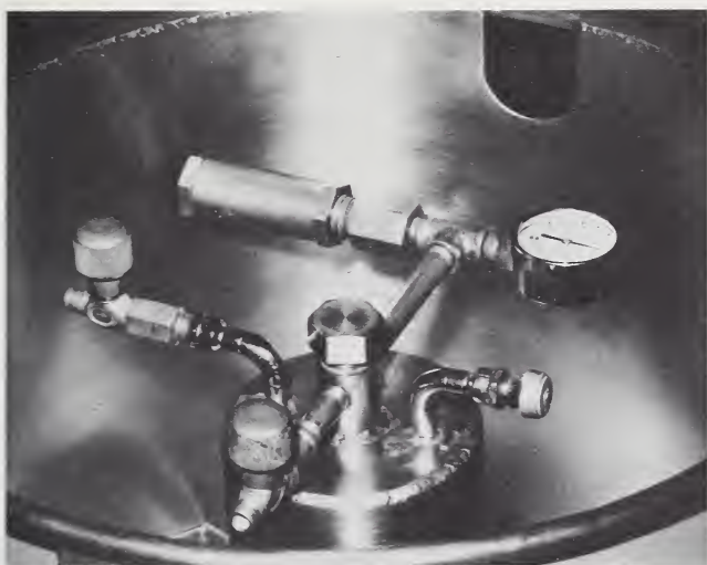
FIGURE 5.22. External view of a typical vapor-shielded helium dewar (Cryogenic Engineering Company), showing access port (center), primary and secondary relief valves, and pressure gage.
