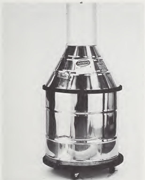
FIGURE 5.3. Typical 25-liter, nitrogen-shielded, liquid helium container ready for shipment.
