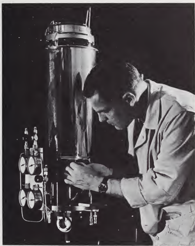
FIGURE 4.46. Gifford-McMahon cycle refrigerator during assembly. (Courtesy of 500 Inc.)
