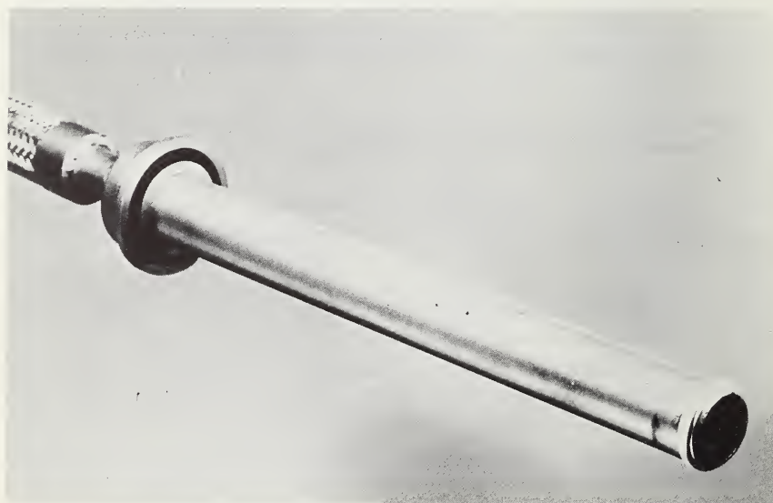
FIGURE 5.34. Liquid helium bayonet, male half, 1- \frac{1}{4} -in diam, 15-in length.
