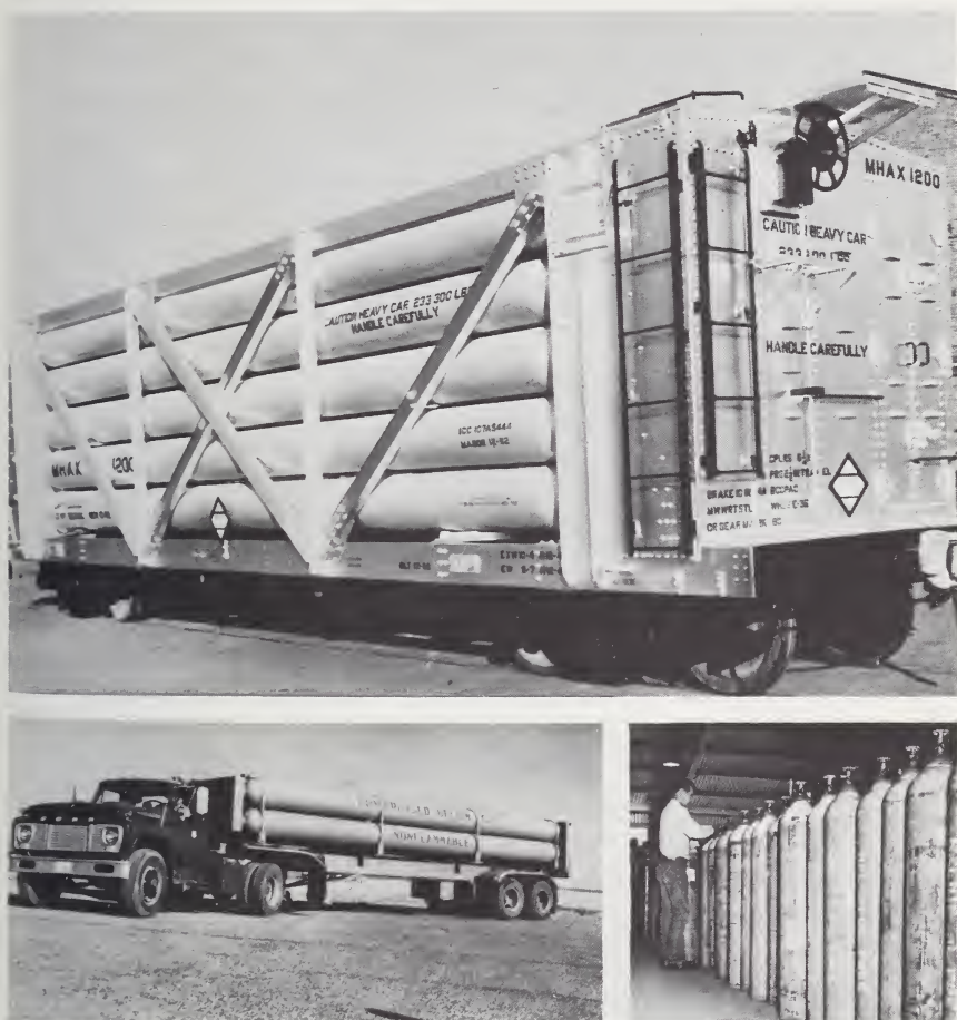
FIGURE 1.13. Equipment used in transporting gaseous helium—railway tank car, highway tube trailer, and standard compressed gas cylinders.
