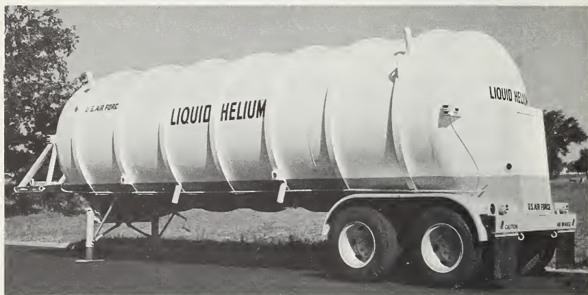
FIGURE 5.9. This 5300-gal semi-trailer, built in 1959, was the first large-scale unit ever constructed for nonvented liquid helium transport.
