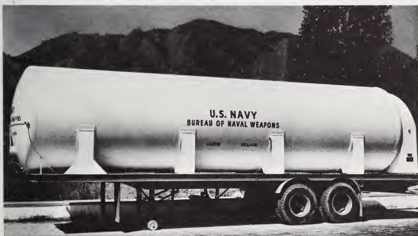
FIGURE 5.8. 7800-gal liquid helium semi-trailer constructed of 5083-0 aluminum by Cryogenic Engineering Company.
