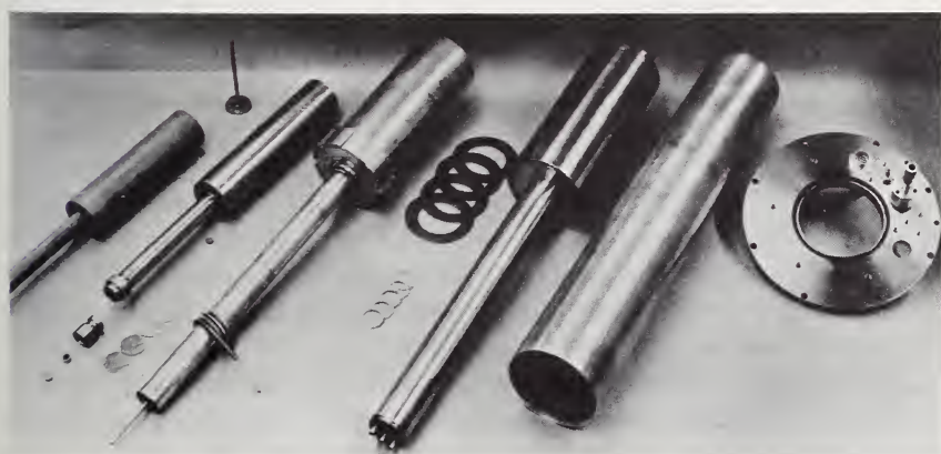
FIGURE 4.30. Internal components of Gifford-McMahon refrigerator.
