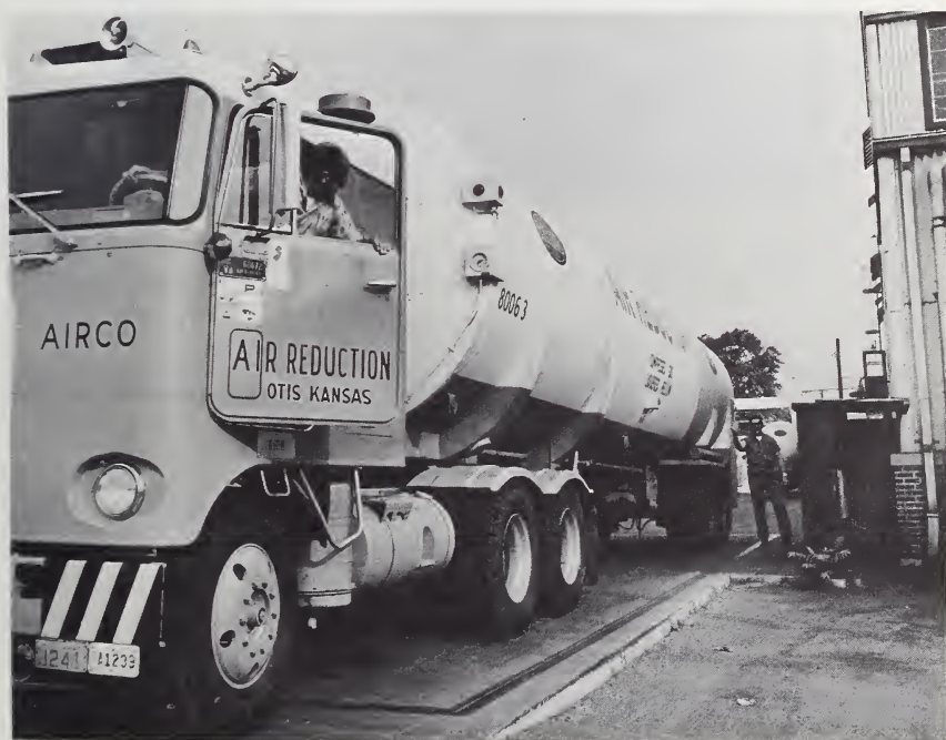
FIGURE 5.49. The 10,000-gal liquid helium semi-trailer is weighed on a truck scale when making custody transfers of its 11,000-lb lading.
